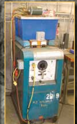
MILLER SR-300-32 WELDER, w/COOLER
